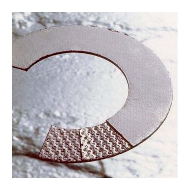
Pure exfoliated graphite with a tanged stainless steel sheet reinforcement for improved blow-out resistance and ease of handling. Due to the excellent chemical and thermal capabilities of graphite it is used extensively throughout the petrochemical and chemical industries for process duties and steam applications.
