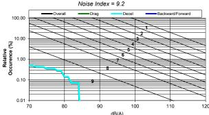
Anti-Noise Shim application for Passenger Car disc brakes. Reduction of brake noise in passenger car disc brakes. The shim serves to reduce the vibrations resulting from the braking process. The construction and design of the shim prevents the brake and axle components from being excited and getting into vibration. These vibrations would lead to the so-called "brake squeal".
